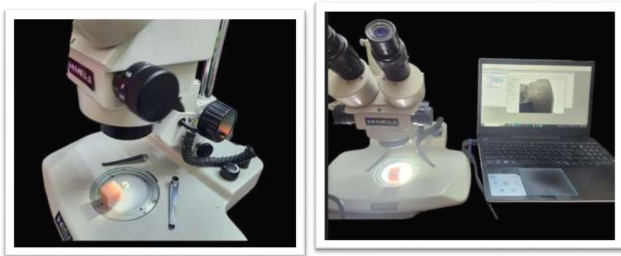
Figure (1): Fracture mode assessment with stereomicroscope under \times 25 magnification
